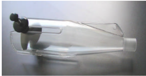
Polycarbonate exposure tube with restrainer
