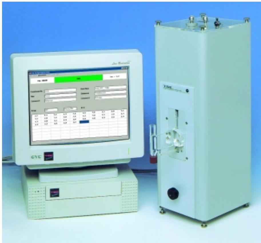
After conversion into volume the numeric values are displayed in user-defined units (ml or  $\mu\text{l}$ ). The data can be printed as a protocol. Data files are generated for further statistical evaluation.
