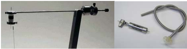
Left: Counterbalance Arm Right: 1-channel fluid swivel with button tether
