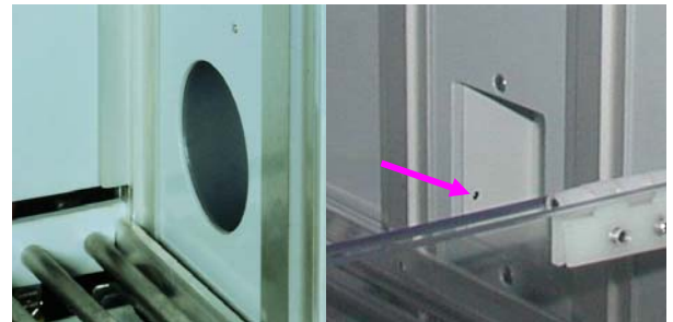
Rat nose-poke modules Left: Circular - diameter 26mm Right: Rectangular with infra-red sensor (arrow)
