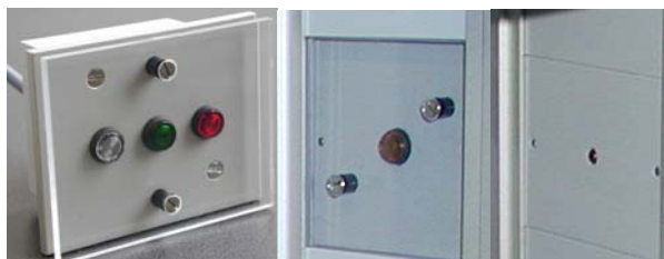
Left: Triple-stimulus lamp set Center: Single red cue lamp Right: Red stimulus LED
