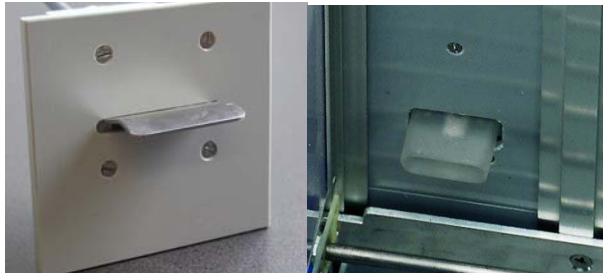
Left: Rat lever module Right: Rat lever with integrated light
