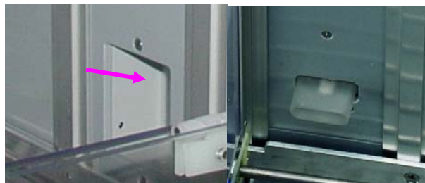
Left: Nose-poke module + integrated lamp (not visible) Right: Rat lever with integrated light
