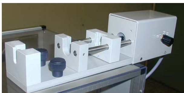
Liquid dispenser ultra-precise, mounted horizontally
