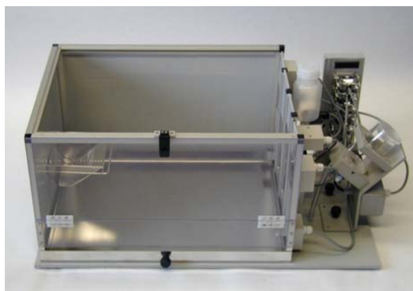
1-panel rat box – fully equipped
