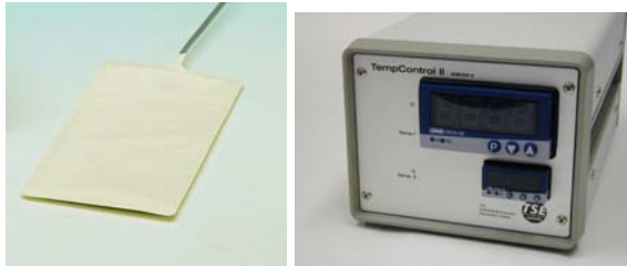
Example: Homeothermic blanket for small laboratory animals
